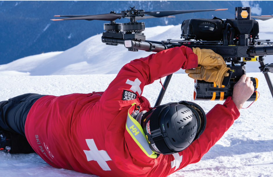
A ski patroller prepares the MONTIS payload on the ground prior to avalanche mitigation.
